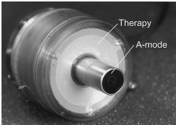
Fig. 1. Transducer configuration used in the simulations and experiments. The outer, spherical-cap transducer has a focal length of 90 mm and an outer diameter of 42 mm. A central aperture houses a coaxial diagnostic transducer with a center frequency of 7.5 MHz, a diameter of 12.5 mm, and a focal length of 60 mm. The diagnostic transducer extends 30 mm out from the apex of the therapy transducer so that the two transducers are confocal.
