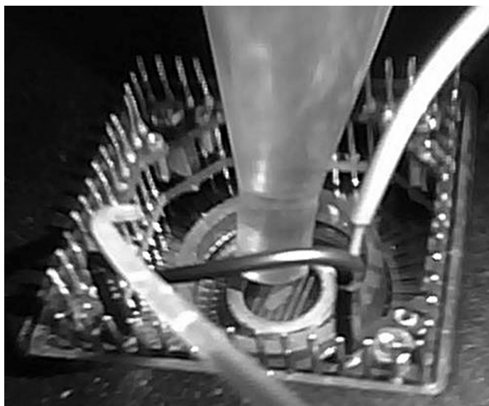
FIGURE 1. Apparatus for functional studies. The tip of the ultrasound coupling cone is immersed in a multi electrode array well. A rat hippocampal slice culture is just below the cone tip. The parallel wires securing the culture are spaced by 1 mm.
