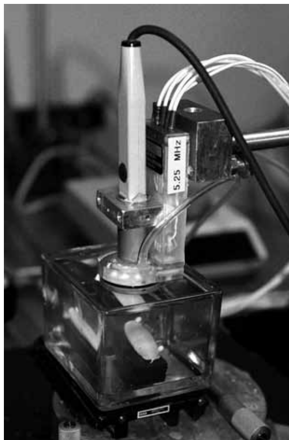
Fig. 1. A 5-annulus Sonic Concepts therapeutic ultrasound transducer was used to ablate bovine tendon ex vivo . Outer diameter was 33 mm and focal length was 35 mm when the elements were in phase. Central frequency was 5.25 MHz and -12 \text{ dB} bandwidth was 45%. A central 14-mm diameter hole admitted a B-K Medical diagnostic array transducer for aiming and monitoring. The transducers are arranged coaxially and confocally. The initial ex vivo tissue model is shown with an unsheathed bovine Achilles tendon pinned to a rubber backing and immersed in PBS. In another set of experiments, the tendon and rubber target were replaced with a layered chicken breast, bovine tendon and glass target.
